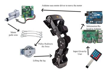
Figure 5: Device Operation
