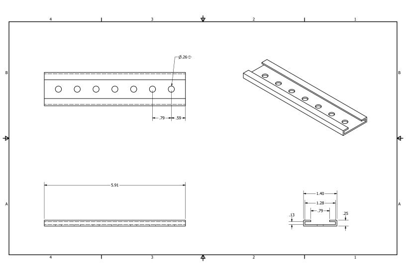
Figure 25: Extension Design in AutoCAD Inventor
