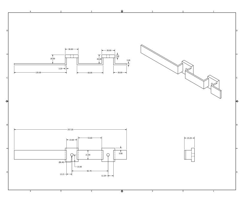
Figure 24: Bracket Design from Sketches in Figure 23 made in AutoCAD Inventor
