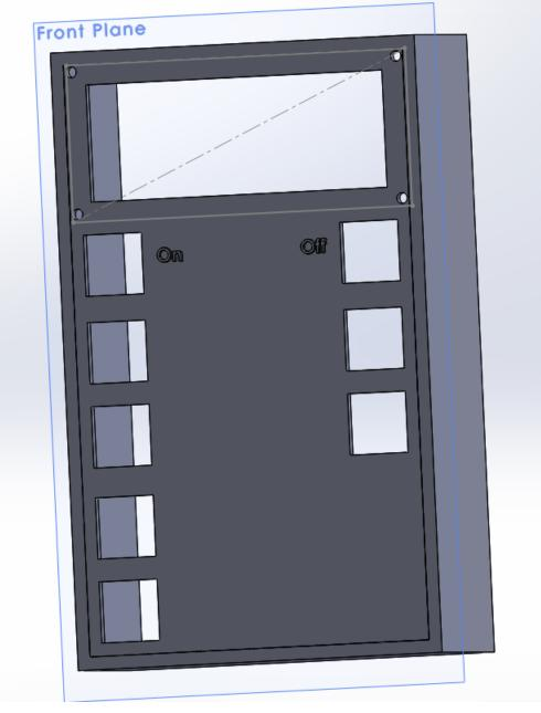
Figure 17: First Semester Controller Body Design Version 3
