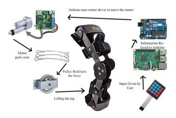
Figure 15: Device Operation
